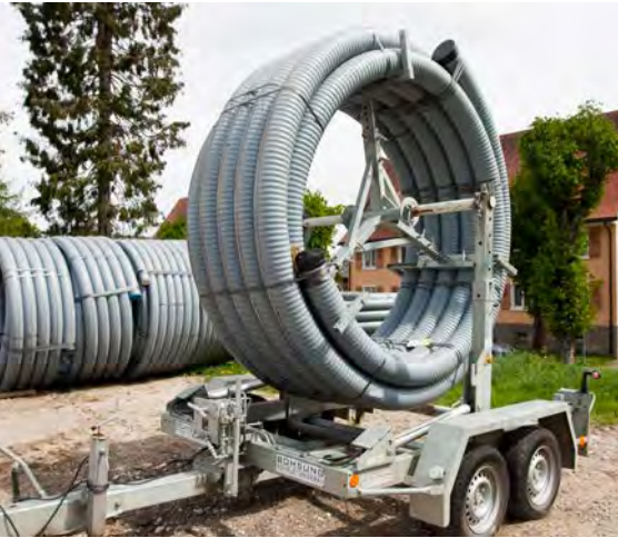
Fig. 07-36 Vertical mobile decoiler
