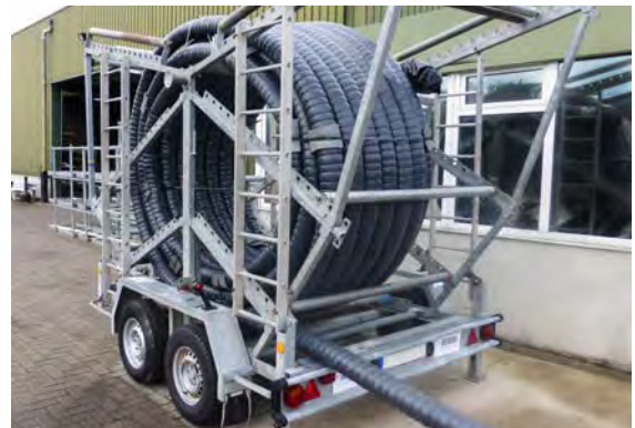
Fig. 07-35 Vertical mobile pipe decoiler
