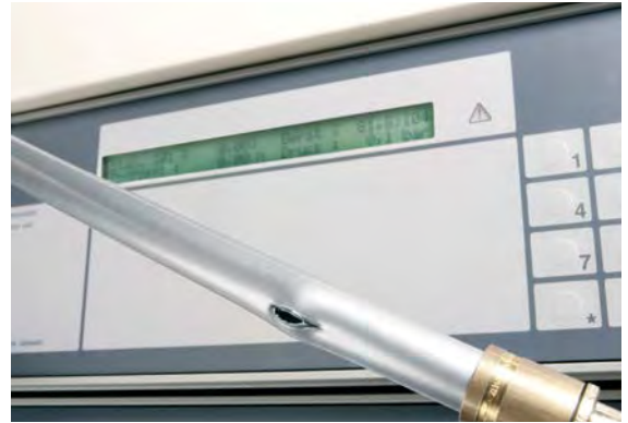
Fig. 03-8 Burst pressure test
